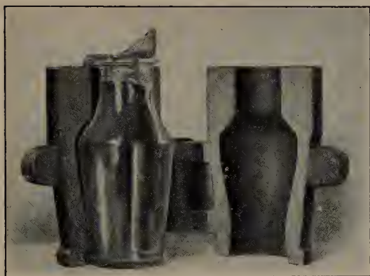
FIG. 149. Making a glass vessel in a mold
